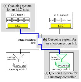
Fig. 10. A two-socket multi-core system and the data path for an LLC miss of CPU node 1 to be served by memory node 2.
