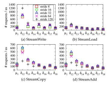
Fig. 8. Measured service rates for the synthetic workloads on the AMD platform for varying stride values.  $\mu_1$  represents the service rate of memory controller 1, and  $\delta_{1\ 2-8}$  represents the service rate of the inter-connection links connecting CPU node 1 and memory controllers 2–8.
