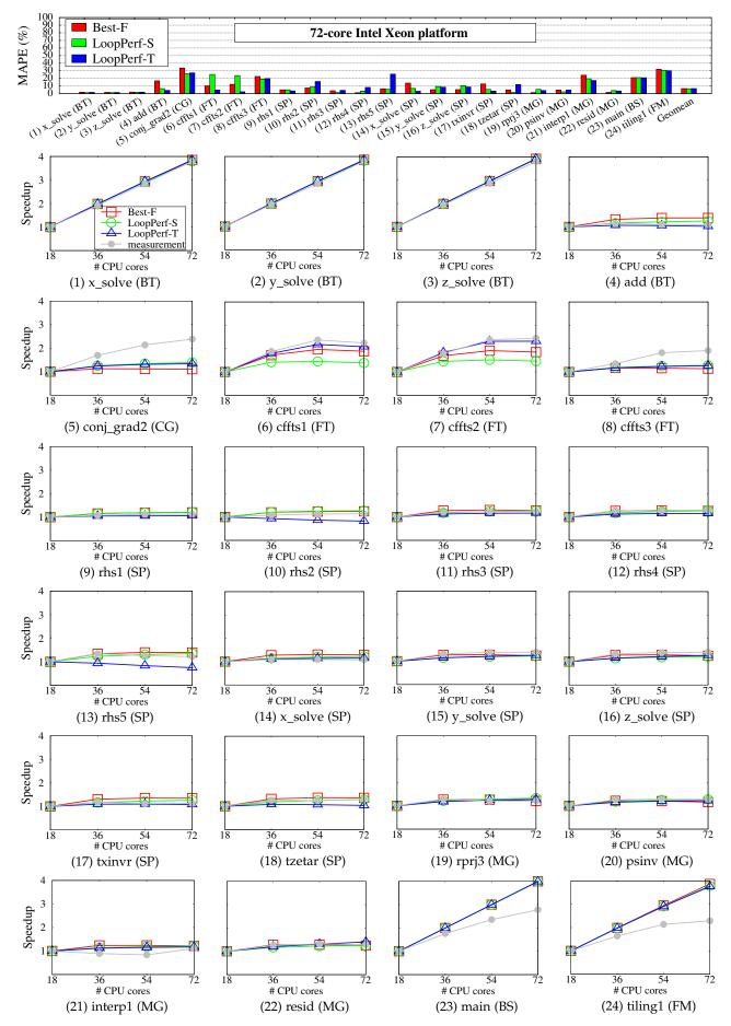
Fig. 13. The predicted speedup and the measured speedup of the parallel loops on the 72-core Intel platform.
