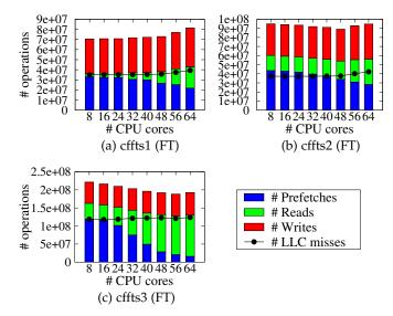
Fig. 6. Number of memory operations of parallel loops for a varying number of worker threads on the AMD platform.
