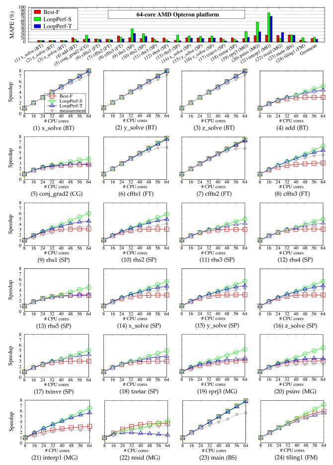
Fig. 12. The predicted speedup and the measured speedup of the parallel loops on the 64-core AMD platform.
