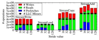
Fig. 7. Number of memory operations of synthetic workloads (using one CPU thread) with different stride values on the AMD platform.
