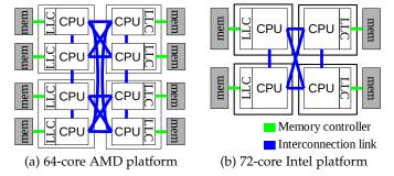
Fig. 3. Block diagram of the target multi-socket multi-core platforms.
