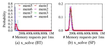
Fig. 4. PMF of the number of memory requests per time for each memory node on the 64-core AMD platform.
